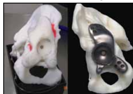
Figure 4: Plastic model of the pelvis with a trial plastic implant seen in the left-hand image. Once the surgeon is happy with the final shape of the implant, the actual implant is manufactured (seen on the right)
